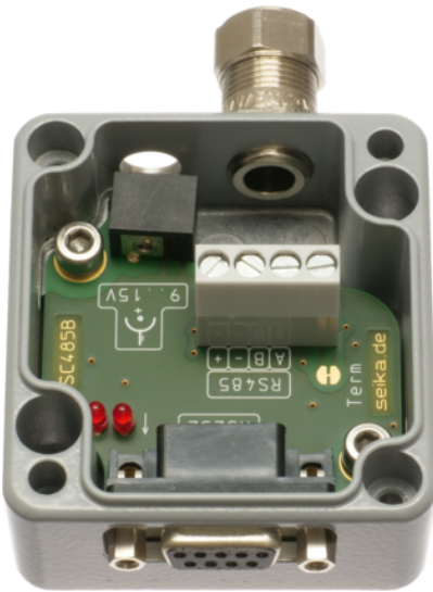
RS232 / RS485 interface converter for connection of SEIKA sensors with RS485 interface to RS232 port of a computer
